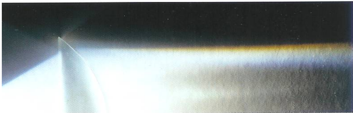
29 Colour defect in a plano-convex lens
